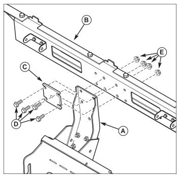
Figure 9. Install Bag and Cover Support
